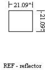
driven and reflector loops are formed from #12 AWG, TW insulated solid copper wire.
